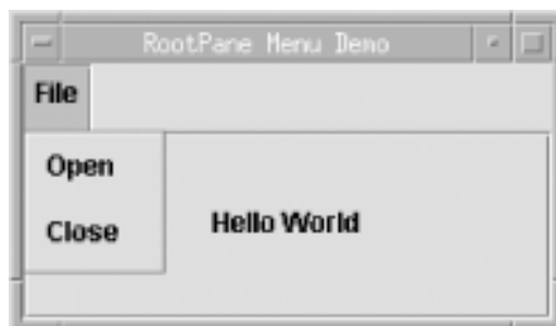
Figure 8-4. JRootPane with a JMenuBar
