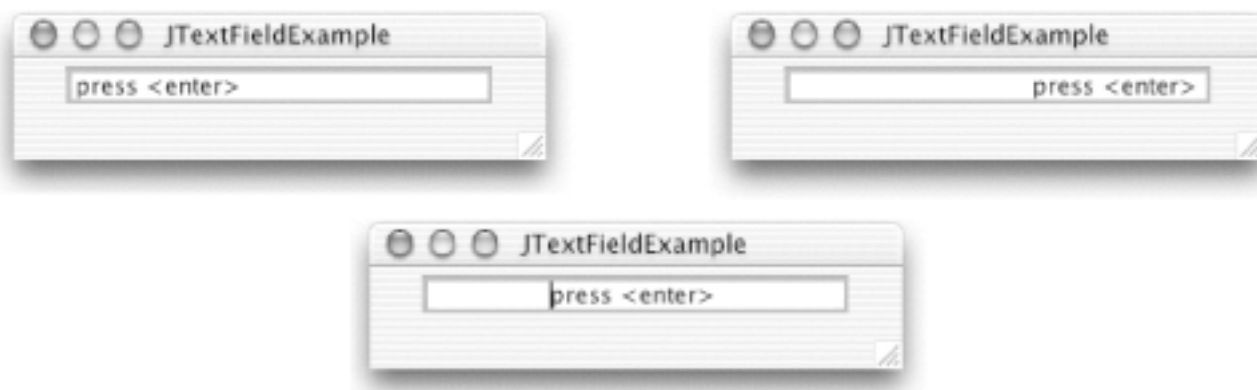
Figure 19-3. JTextFields shown with different alignments
