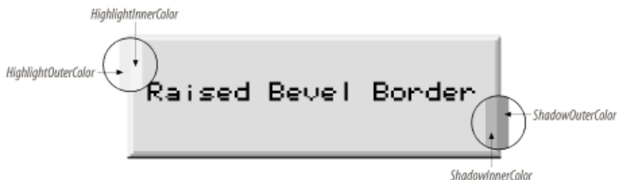
Figure 13-5. The four colors of a bevel border
