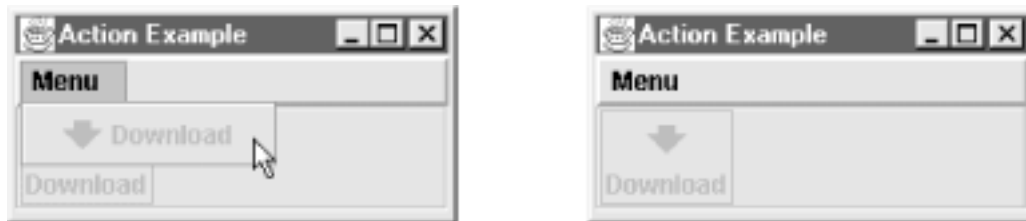
Figure 3-3. A disabled action in a menu and in a toolbar
