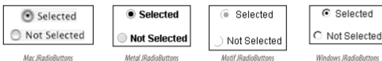
Figure 5-8. JRadioButtons in four L&Fs
