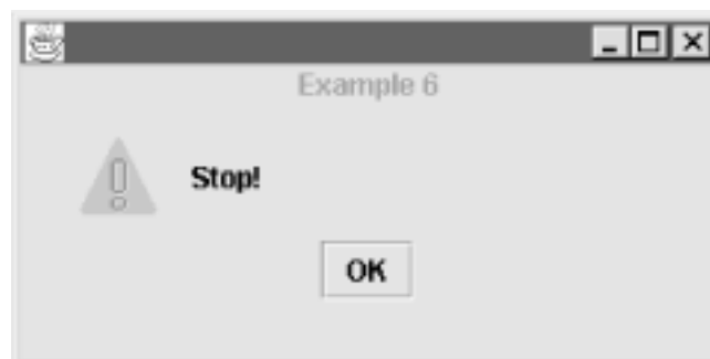
Figure 10-13. A JOptionPane inside a Swing container
