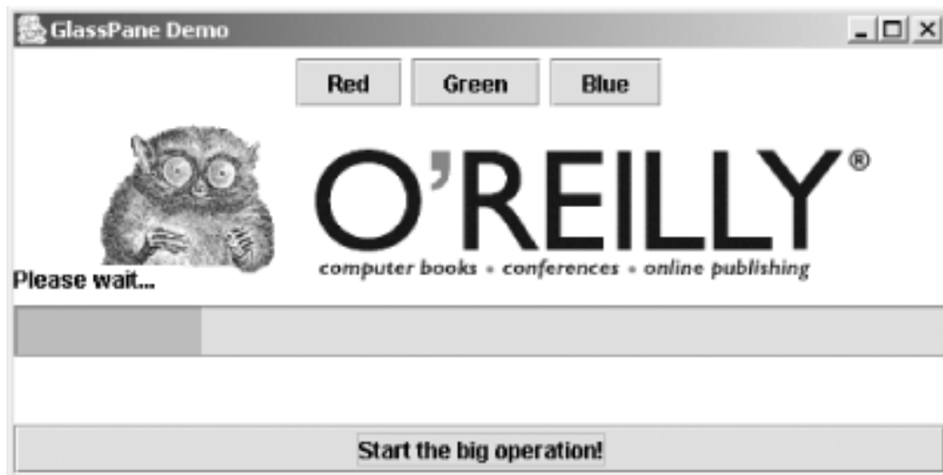
Figure 8-5. JRootPane with an active glass pane (which contains the progress bar)
