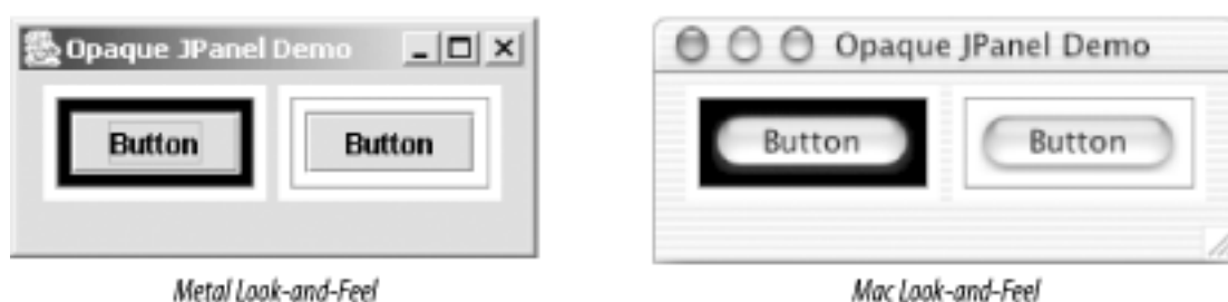
Figure 8-1. Opaque and nonopaque JPanels (in Metal and Mac L&Fs)
