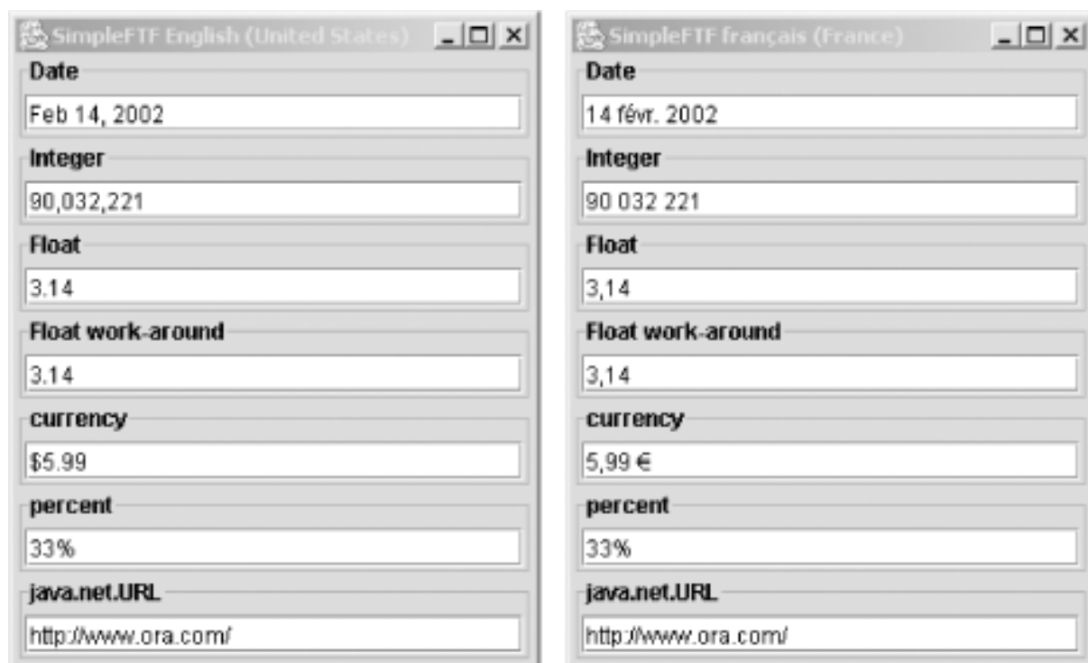
Figure 20-1. JFormattedTextFields in two different locales
