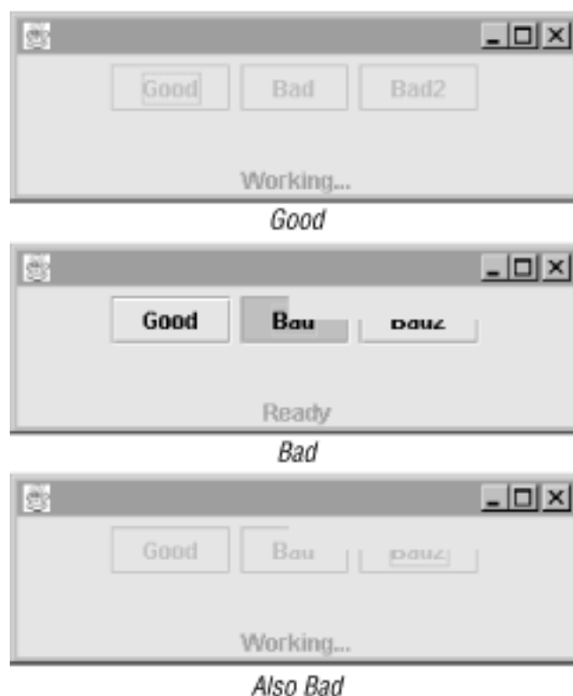
Figure 28-5. Correct and incorrect management of the event dispatch thread
