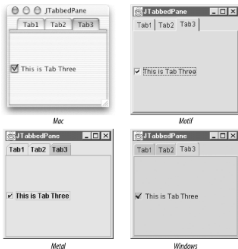
Figure 11-7. A simple tabbed pane with three tabs in several L&Fs
