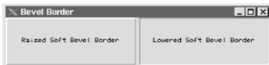
Figure 13-6. Soft bevel borders in Swing
