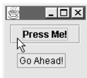
Figure 3-8. A tooltip for a component
