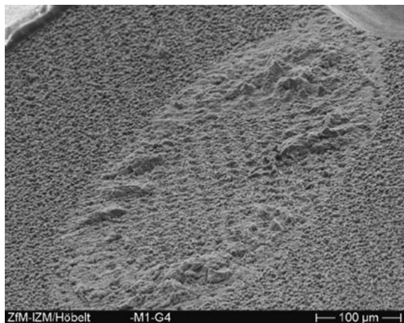
Fig. 11.45 Lift-off pattern as a result of power cycling
