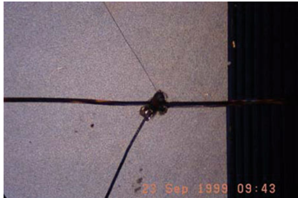
Fig. 12.19 Failure picture of a diode destroyed by dynamic avalanche of the third degree
