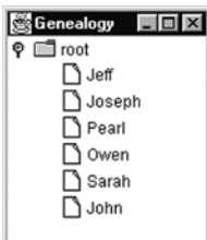
Figure 8-5. In this example, the root node appears because you've explicitly indicated it should be displayed
