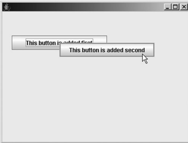
Figure 6-44. Once the cursor is moved over the “second” button, it appears to be on top of the “first” one
