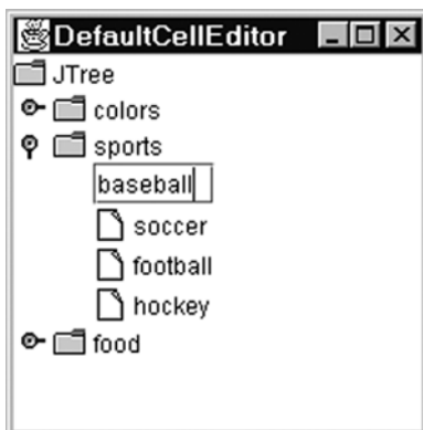
Figure 8-20. Double-clicking a tree cell with editing enabled causes a text field to appear in which the cell's text representation is displayed and can be edited
