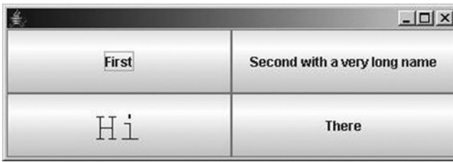
Figure 6-6. GridLayout distributes both horizontal and vertical space evenly to the components regardless of their preferred sizes
