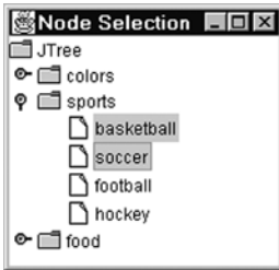
Figure 8-26. How a JTree appears when the basketball and soccer nodes are highlighted
