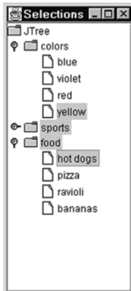
Figure 8-30. In this example, the children of the sports node aren't considered to be selected because their parent is collapsed
