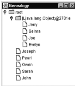
Figure 8-6. Defining a node as an array results in the array elements being represented as children within the tree
