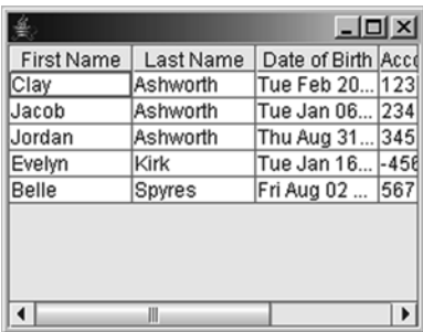
Figure 7-7. Changing the auto resize mode results in a scrollbar appearing when the table isn't wide enough to display the contents of all its columns
