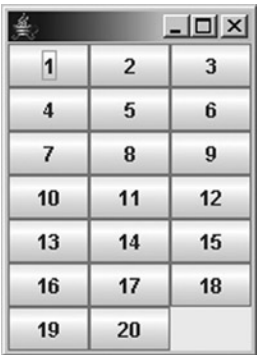
Figure 6-7. You can force GridLayout to use a specific number of columns by specifying a column count but no row count
