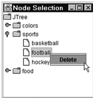
Figure 8-32. You'll often want to allow users to perform operations on the selected node(s) in a tree, and getSelectionPaths() can be helpful when doing this
