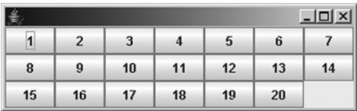
Figure 6-8. You can force GridLayout to use a specific number of rows by specifying a row count but no column count
