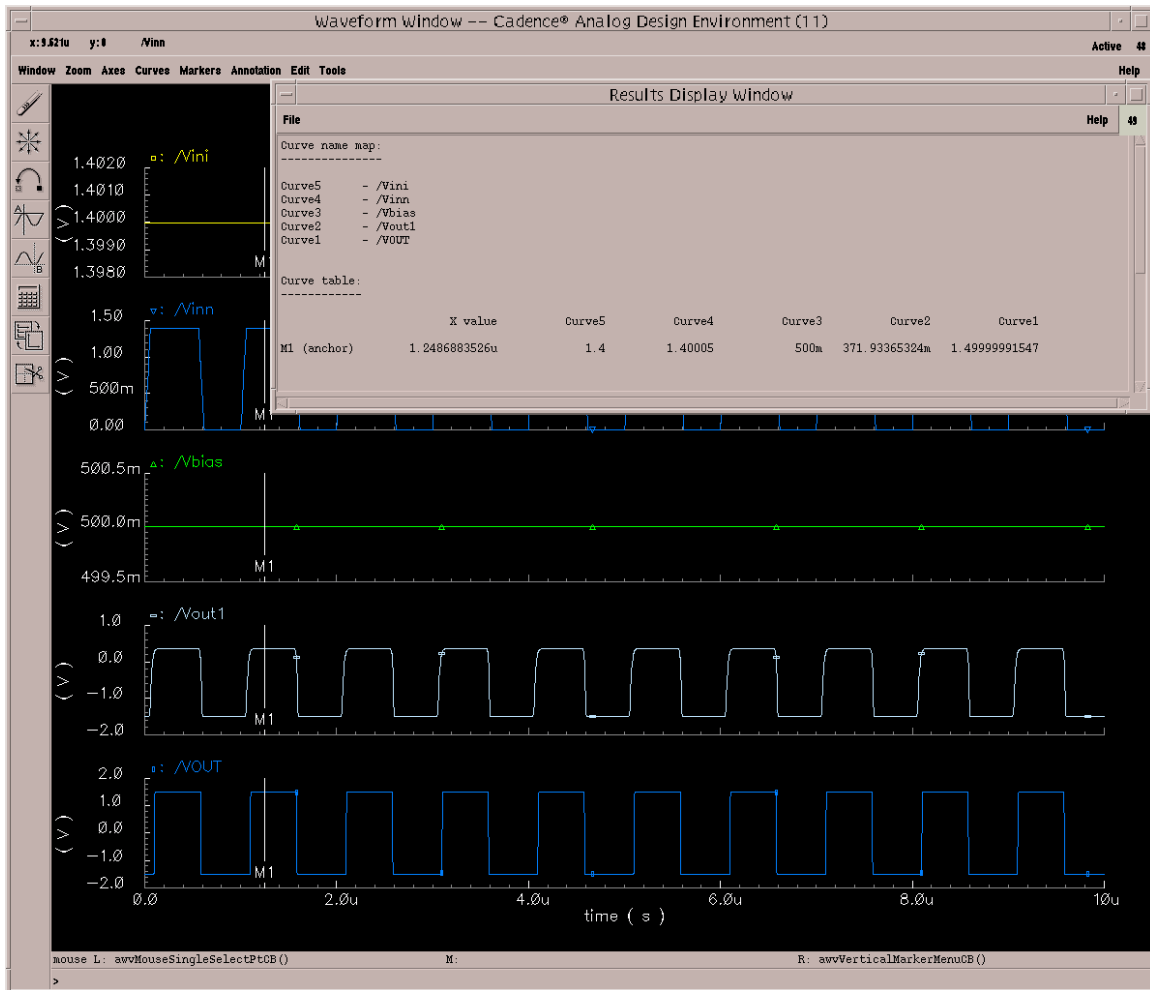
Figure 18: Gain of the op-amp with W7=17.
