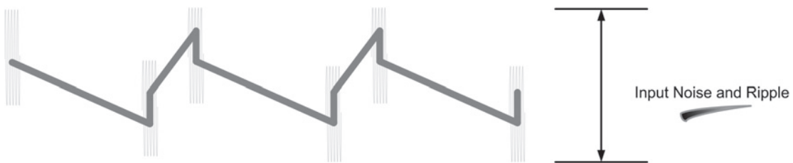
Figure 2-8 Typical Input Noise and Ripple Waveform of a Buck (AC Component Only)
