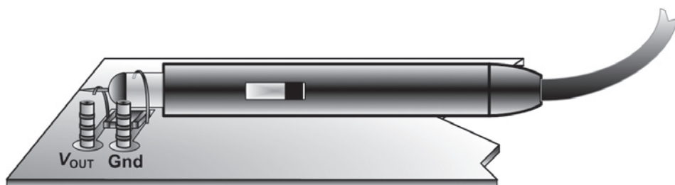
Figure 3-4 Correct Way to Measure Output Noise and Ripple
