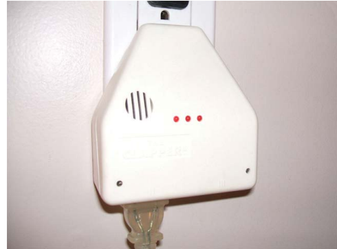
FIGURE 14-1: A clapper plugs into the wall and controls turning on and off an electrical socket.
