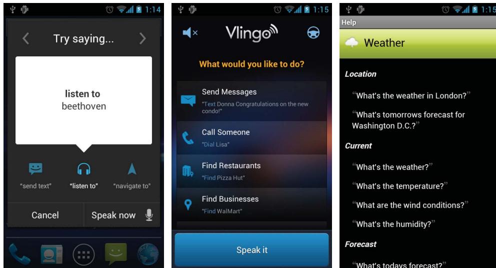
FIGURE 15-4: Three help screens from Google Voice Search, Vlingo, and Edwin show different ways to explain to users what they can say.
