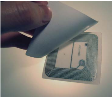
FIGURE 11-1: The internal components of an RFID sticker
