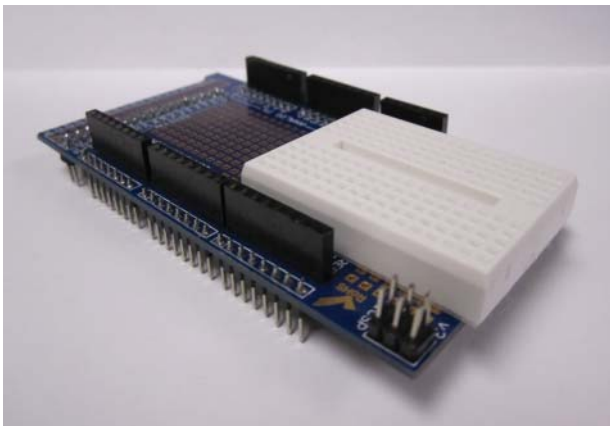
FIGURE 10-3: An Arduino Mega “breadboard” shield. Shields interface with the pin headers and sit atop a microcontroller board. Sensors or other devices may sit on a shield.
