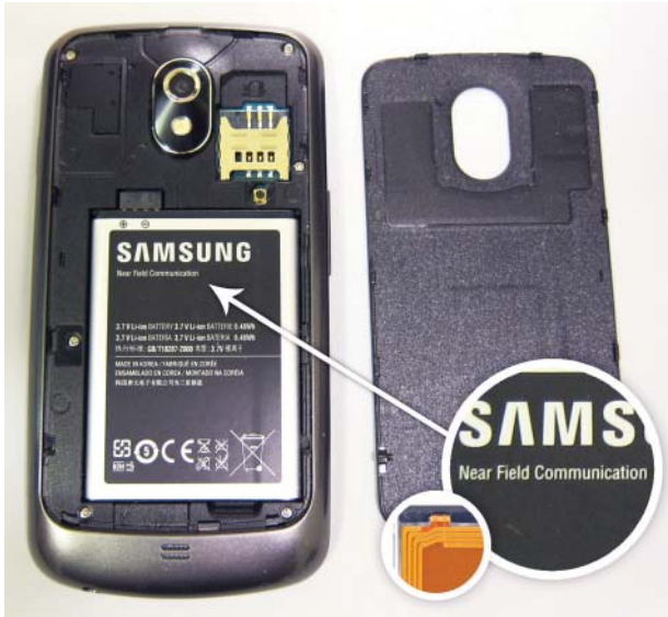
FIGURE 11-4: The NFC antenna on the Galaxy Nexus comes as part of the battery (right).
