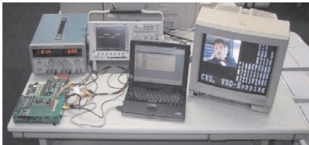
(b) Fig. 4.66 (a) Power dependence on workload. (b) V_{DD} -hopping system.
