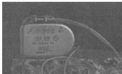
Figure 1-4. Pacemaker manufactured by CCC del Uruguay S.A. ([CCC03]), showing the titanium case and the epoxy "neck" where leads are connected.
