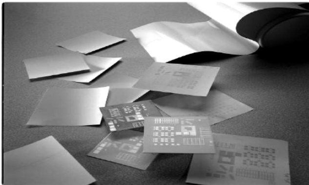
Figure 14-4. Unfired (“Green”) Ceramic Tape
