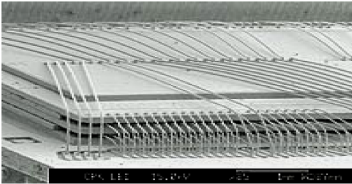
Figure 5-13. SEM of a 4 Stacked Die Assembly with 2 Spacers
