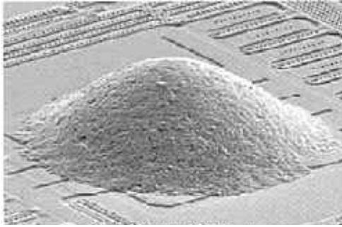
Figure 10-16. Stencil Printed Conductive Epoxy Bump (75 \mu m)
