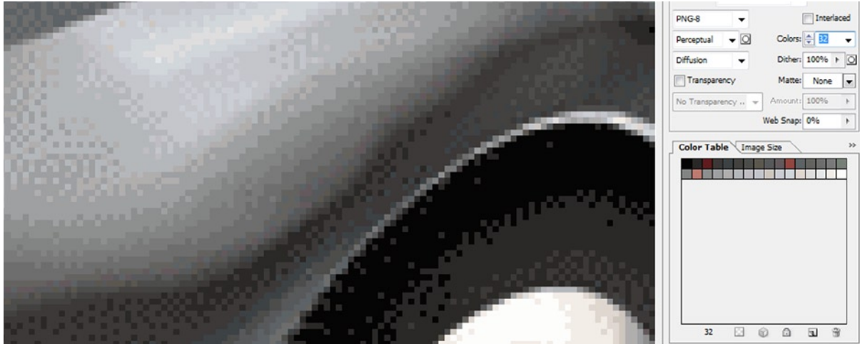
Figure 9-3. The dithering effect in an indexed color image with compression set to 32 colors (5-bit color)
