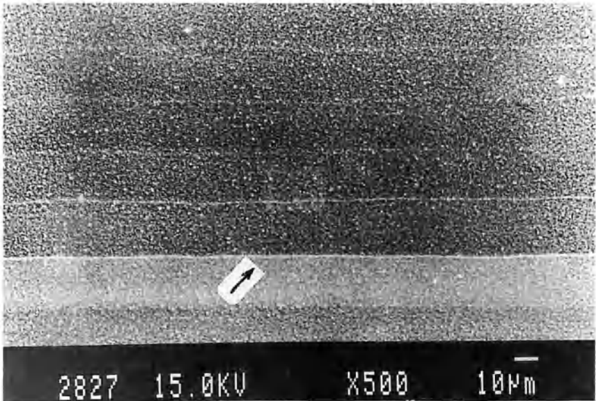
Figure 3. Localized subboundaries formed under action of periodic thermal relief.
