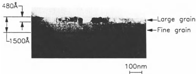
Fig. 5. Cross-sectional TEM micrograph of laser crystallised PECVD Si.
