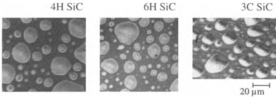
Figure 2: Blistering effects in three SiC polytypes after H ion implantation at the same dose and energy.
