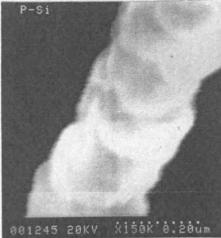
Figure 4. Whisker with semi-spherical nuclei arranged periodically on external surface.
