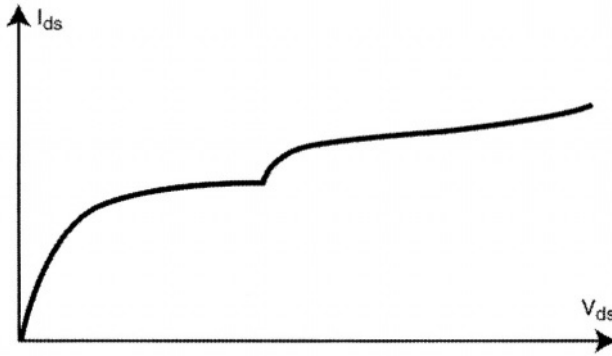
Figure 2.13: Graph showing the kink effect. As source-drain voltage is increased, the output current passes through the impact ionization threshold region, and output current is boosted.
