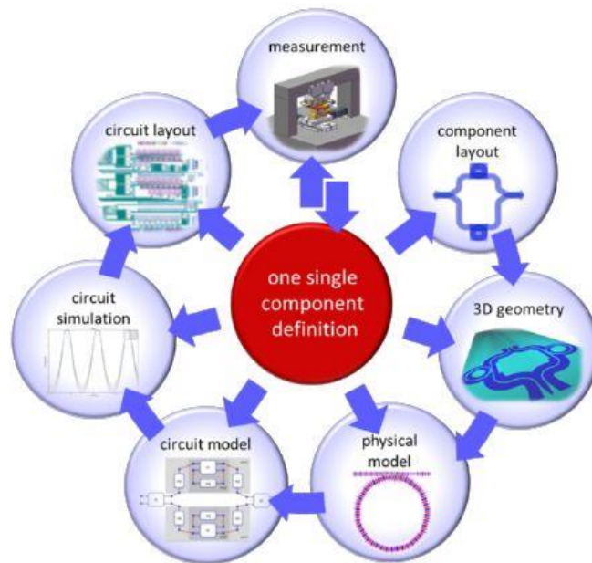
Figure 8. The IPKISS design framework where the design flow is oriented to the definition of single components with different views used for different design stages. [97]
