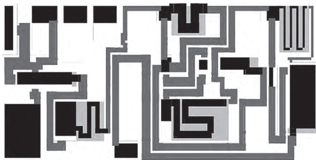
FIGURE 19.3 Microwave frequency (~60 GHz) device-level floorplan shows devices, planar wiring on a single layer, and several instances of “detours,” which are inserted to match lengths and electrical properties of wires in this small design. (From Aktuna, M. et al., IEEE Trans. CAD , 18, 375, 1999. With permission.)
