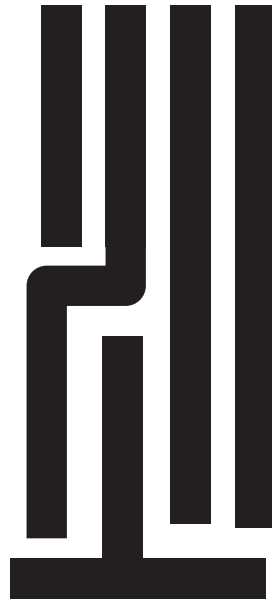
FIGURE 21.25 Layout structures that represent topologies leading to “phase conflicts.”
