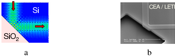
Fig. 9. Etched mirror for 90° turn of rib waveguides: FDTD calculation of the field amplitude (a) scanning electron microscope (SEM) view after removal of the silicon oxide (b).
