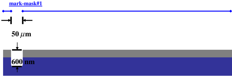
Fig. 11.20. Alignment mark formation.
