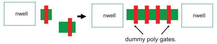
Fig. 14. Reducing layout-induced variability by following layout guidelines.
