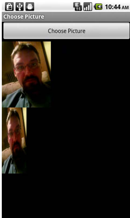
Figure 3–5. The second image displayed with the custom matrix applied, scaling the x axis by 50%
