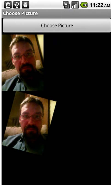
Figure 3–14. Matrix applied when Bitmap created; the dimensions of the Bitmap are adjusted to match the actual image data.
