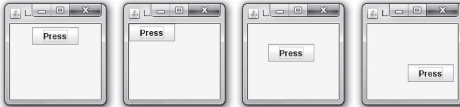
Figure 16-4 Execution of the JDemoLocation program
