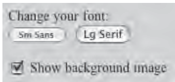
B The buttons and check box are browser objects, which can be manipulated by JavaScript.
