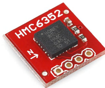
Figure 13.8: HMC6352 mounted on a breakout board. (Image reproduced with permission of Sparkfun Electronics)
