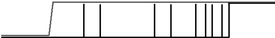
FIGURE 9.10: Contact bounce. The gray signal represents when the switch is pressed and the black represents the output conductance (open circuit to close).
