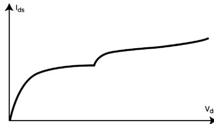
FIGURE 6.4: Kink effect in PDSOI: the parasitic NPN can turn on, discharging the floating body, but sourcing current from drain (collector) to source (emitter).
