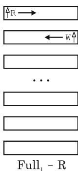
Fig. 9-9. Register addressing for an almost-full FIFO.
