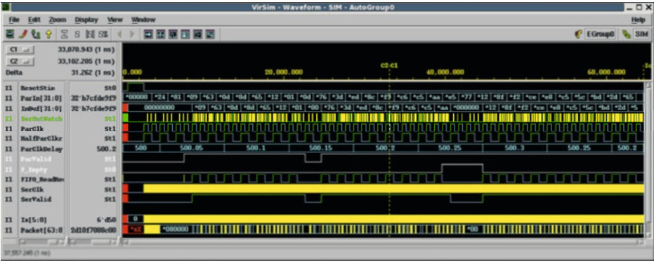
Fig. 21-13. Overall view of synthesized PLL netlist simulation.
