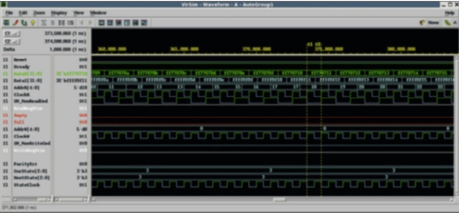
Fig. 21-16. Zoomed-in view of synthesized FIFO netlist simulation, showing individual 32-bit word transfers.
