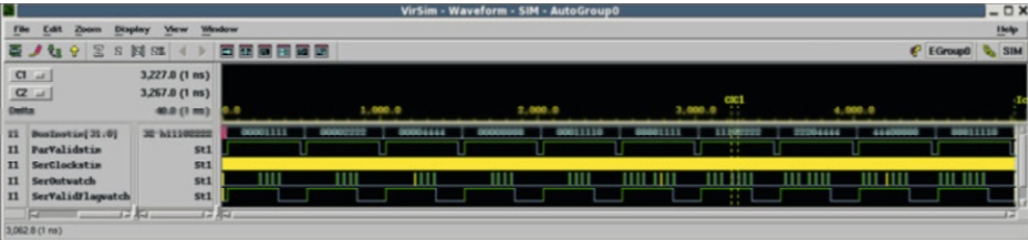
Fig. 5-14. Overview simulation of the generic parallel-to-serial converter.
