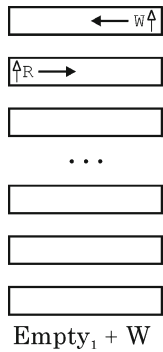
Fig. 9-5. Register addressing for an almost-empty FIFO.
