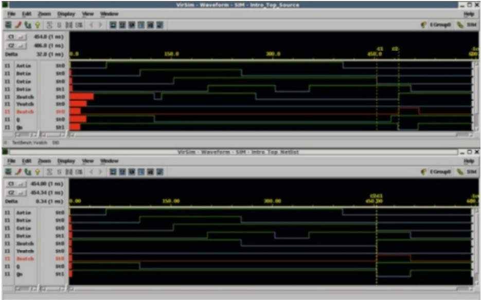
Fig. 23-2. Timing differences between the verilog source (above) and its synthesized netlist.
