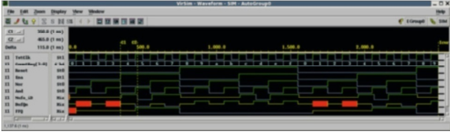
Fig. 17-6. SpecIt simulation with distributed delays.
