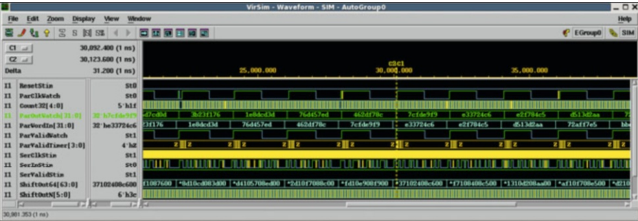
Fig. 21-18. DesDecoder netlist simulation, zoomed in to resolve individual parallel-bus words.
