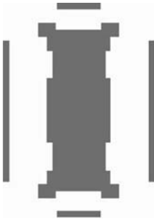
Fig. 3.25 Optical proximity correction (OPC) and SRAFs applied to a layout (adapted from [51]).
