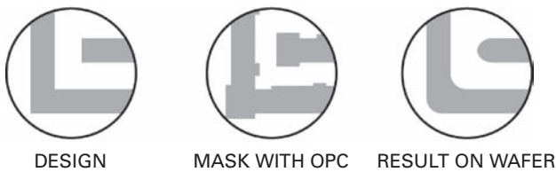
Fig. 3.24 Optical proximity correction (OPC) counteracts lithography distortions (adapted from [48]).
