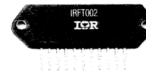
Figure 17.9. Hybrid MOSFET package for motor control. (Courtesy of International Rectifier Corp.)
