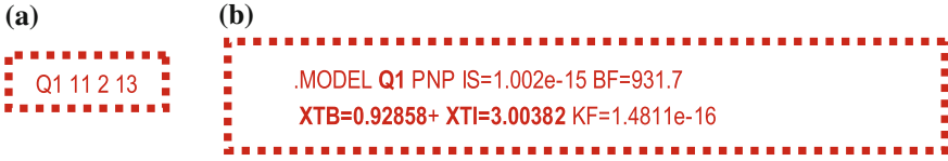
Fig. 7.7 Declaration of one of the two transistors in the op-amp SPICE model
