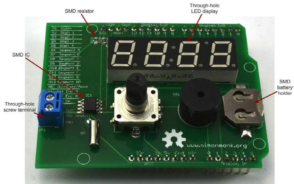
FIGURE 1-2 Through-hole and surface-mount components.
