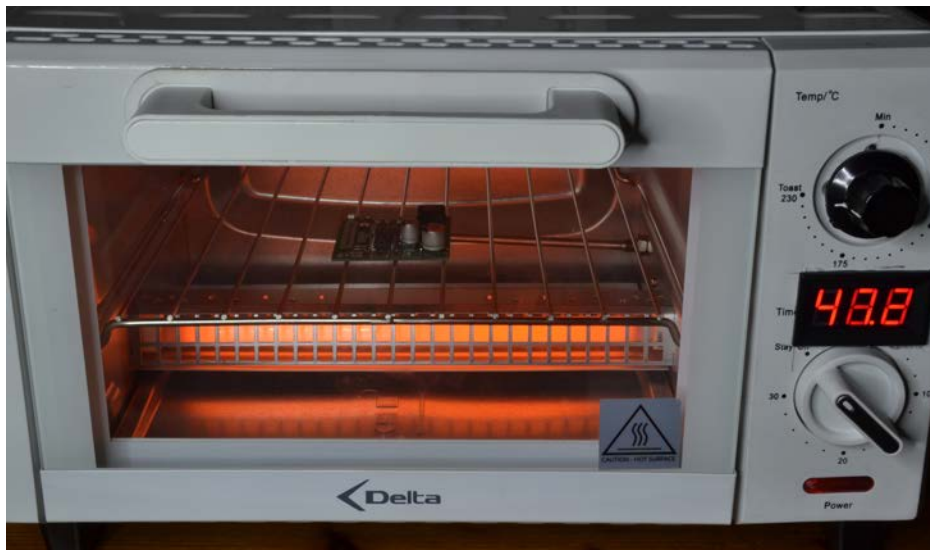
FIGURE 7-20 Cooking the board.
