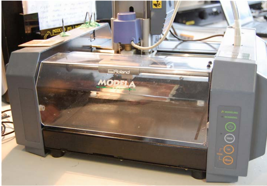
FIGURE 6-6 CNC router cutting a PCB.
