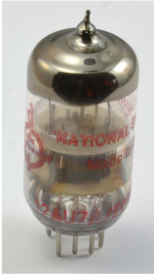
FIGURE 11-7 A 12AU7 triode tube.
