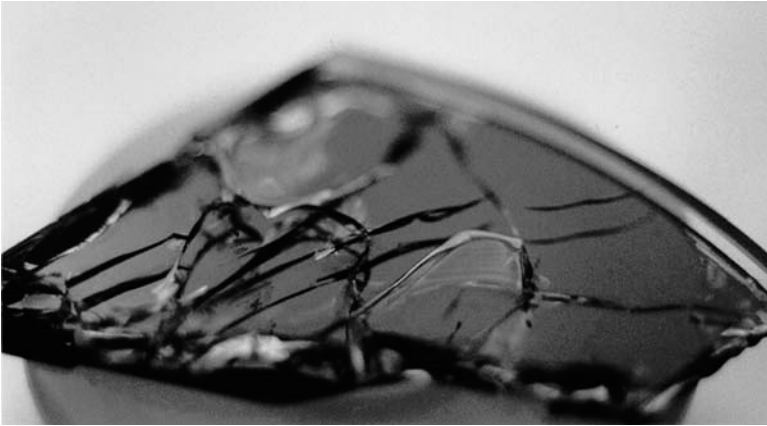
Fig. 4.37. Fracturing of thermally mismatched silicon and Palex sodium glass ( \alpha_g = 6 \cdot 10^{-6} \text{ K}^{-1} ) sandwich, bonded anodically, observed after cooling down of the sample from 400^\circ\text{C} to 20^\circ\text{C} .
