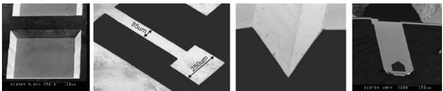
Fig. 3.40. Silicon three-dimensional, wet anisotropically etched microconstructions: membranes, seismic mass suspended on beams, V-groove, sharp tip at a beam.
