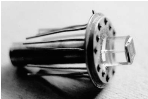
Fig. 4.120. 20 kPa silicon pressure sensor die on a glass column.
