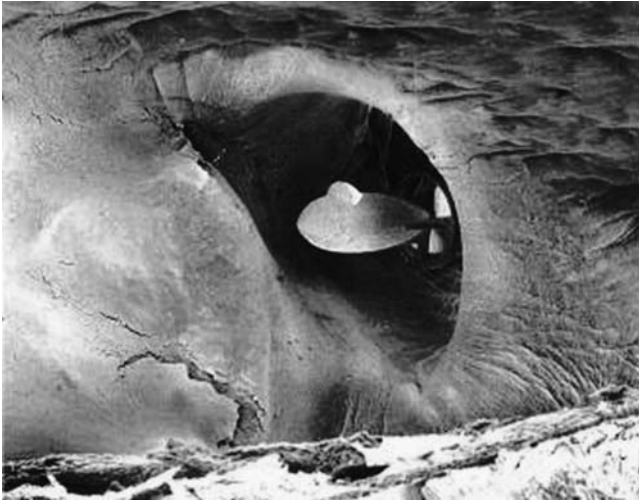
Fig. 5.4. Miniature submarine with the dimensions of about 4\text{ mm} \times 0.8\text{ mm} sailing in a blood vessel. The rotating screw powered by an electric microengine drives the hull; it can be equipped with a TV camera and different sensors (by courtesy of the Micro-TECH Co., Duisburg, Germany).
