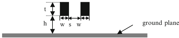
Fig. 9.10 The cross section of a two-parallel-wire structure (Reprinted with permission from Yu et al. [186] © 2012 Elsevier)
