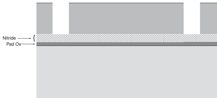
Figure 4-6: Resist Pattern for Trench Etch
