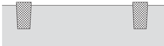
Figure 4-2: Shallow Trench Isolation Cross Section
