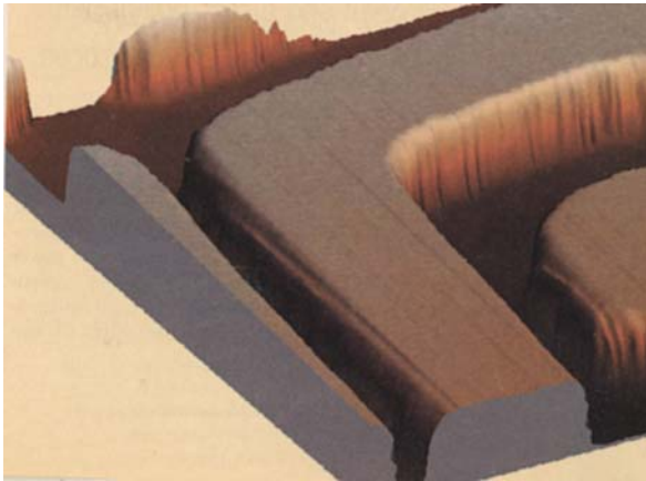
Fig. 6.22 A stylus nanoprofilometry image of an STI region (Reproduced with permission, Semiconductor International, March 2000, p. 71)
