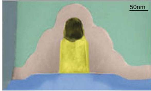
Fig. 4.3 Scanning electron microphotograph of one of the 58 million transistors fabricated on a single chip following 130 nm-node technology. The interconnections are made out of copper (Photo courtesy, IBM, Research, G-5 processor)
