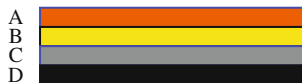
Fig. 3.16 A stack of films deposited following the damascene process. A is copper, B is the barrier layer, C is the dielectric, and D is silicon
