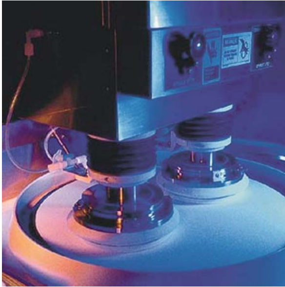
Fig. 6.15 A commercial CMP machine with polishing head and the attachments (Reprinted with permission, Semiconductor International, Nov. 1998, p. 57)
