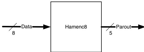
Figure 7.18 An 8-bit Hamming code encoder.
