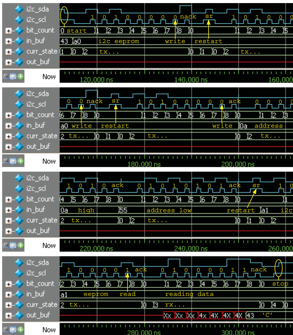
Figure 14.49 Waveform of I2C EEPROM read
