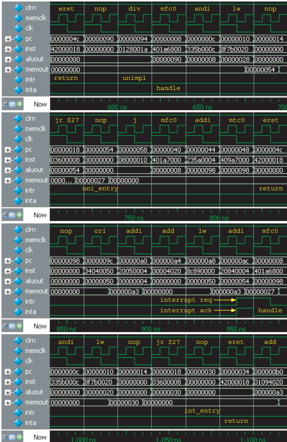
Figure 6.13 Waveform of unimplemented instruction exception and interrupt
