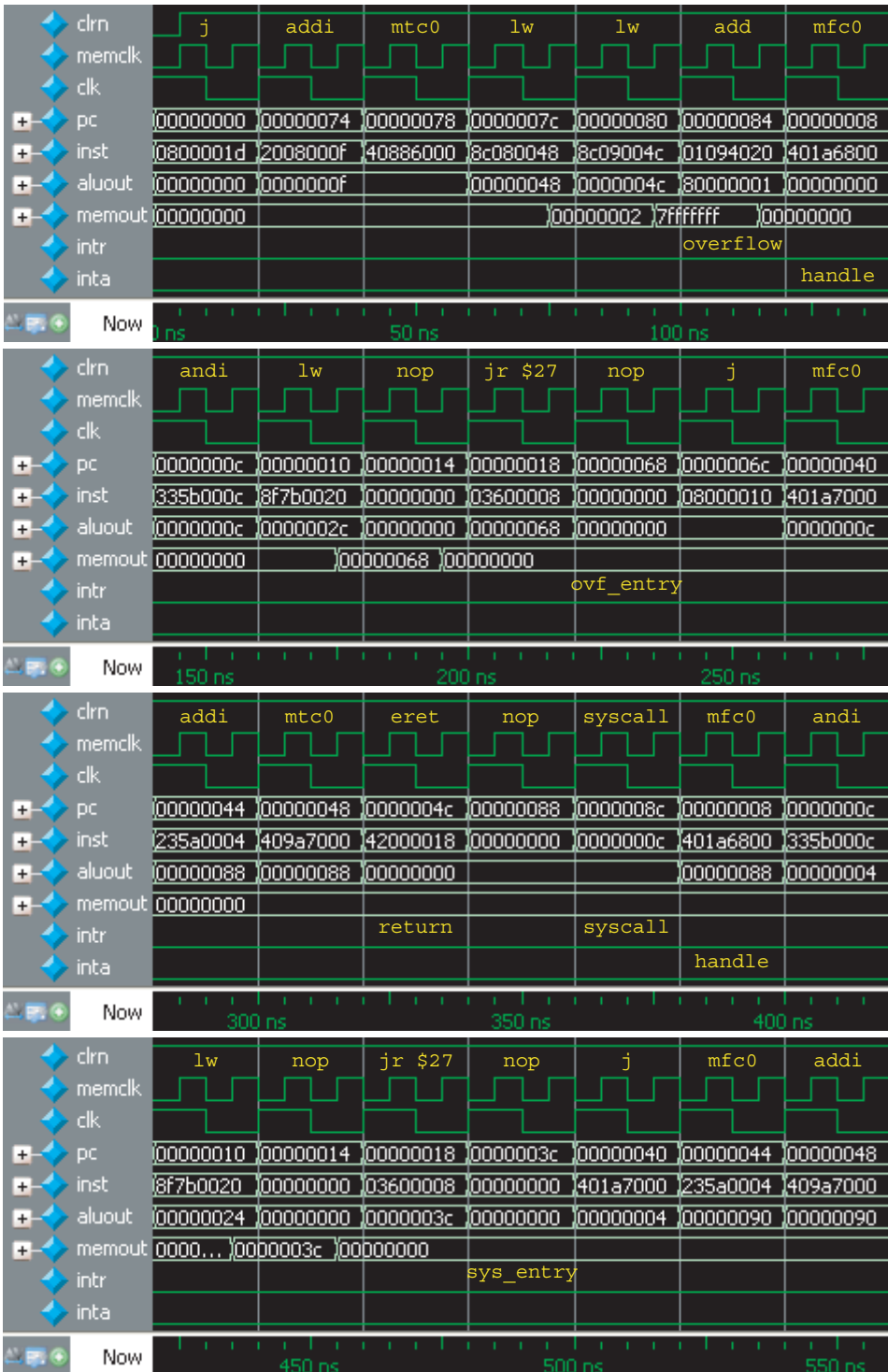
Figure 6.12 Waveform of overflow and system call exceptions
