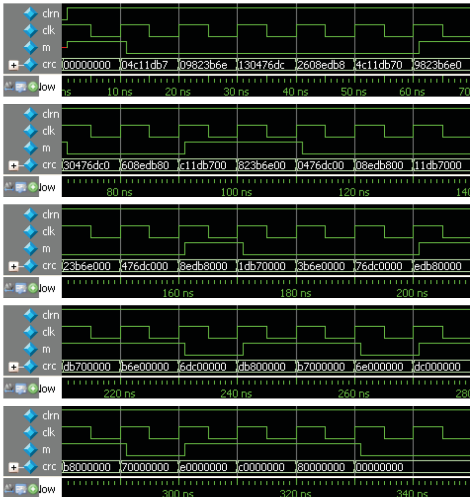
Figure 14.11 Waveform of CRC-32-IEEE calculation circuit
