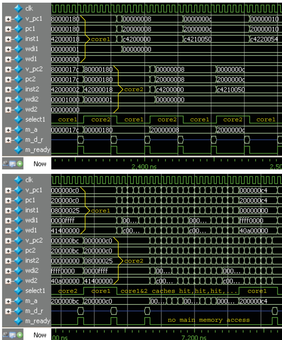
Figure 13.15 Waveform of a dual-core CPU (caches hit)
