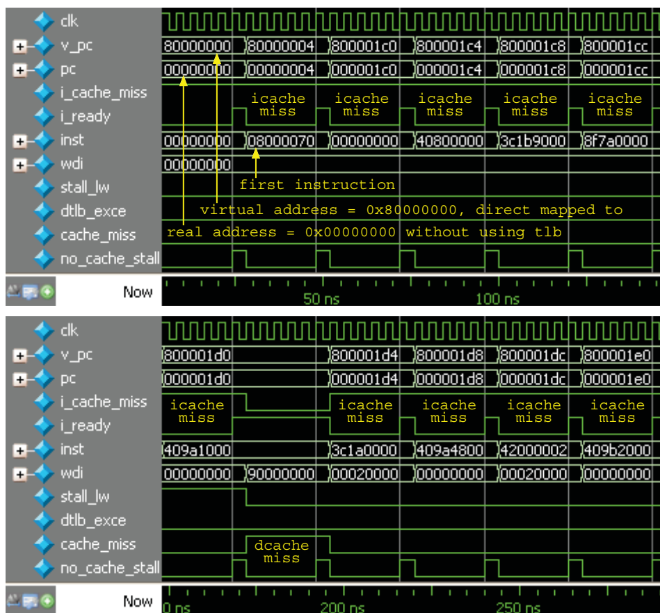
Figure 12.18 Waveform of initializing ITLB
